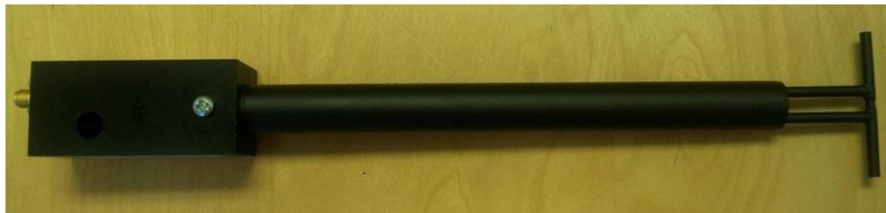
Figure 1 – MVG COMOSAR Validation Dipole
