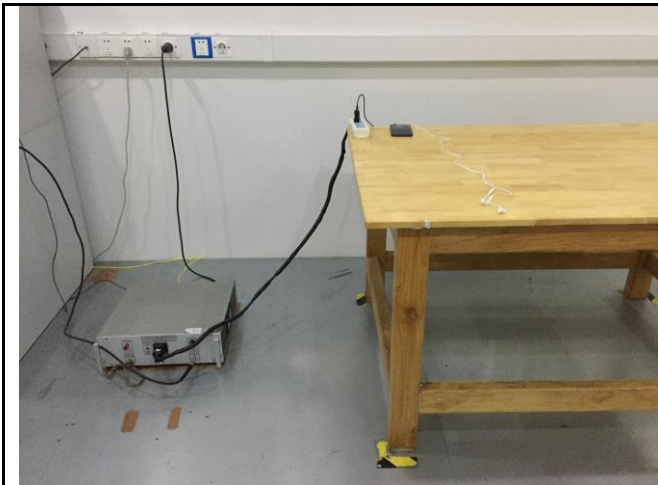
Conducted Emissions Test Setup Front View
