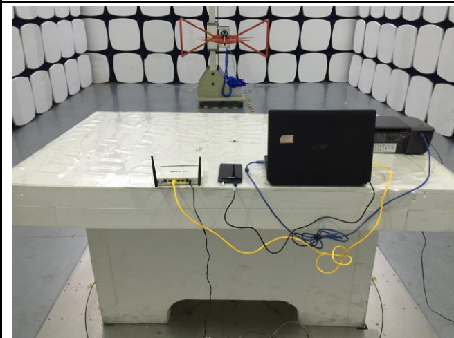
Radiated Emissions Test Setup Below 1GHz
