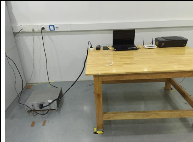
Conducted Emissions Test Setup – Front View
