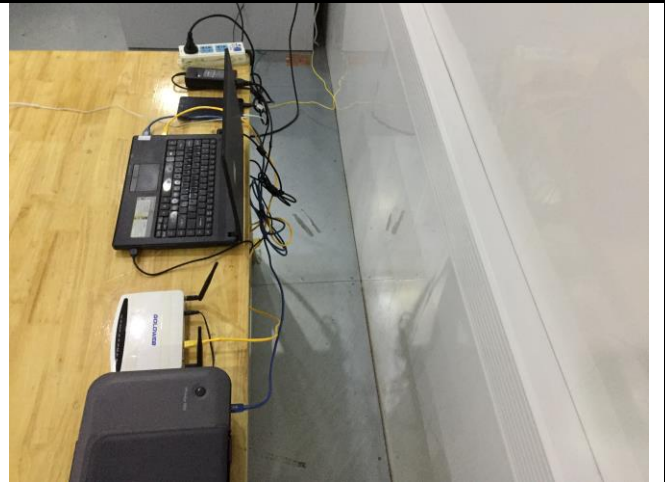
Conducted Emissions Test Setup – Side View
