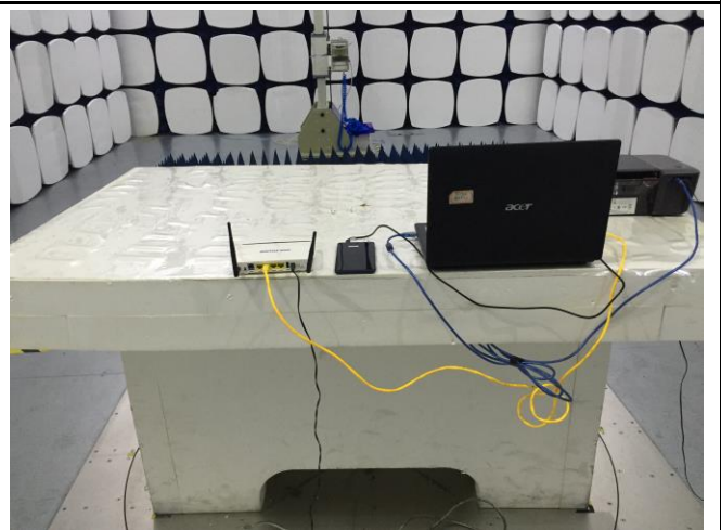
Radiated Emissions Test Setup Above 1GHz
