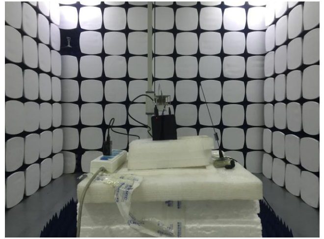
Radiated Spurious Emissions Test Setup Above 1GHz
