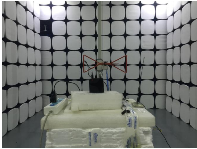
Radiated Spurious Emissions Test Setup Below 1GHz
