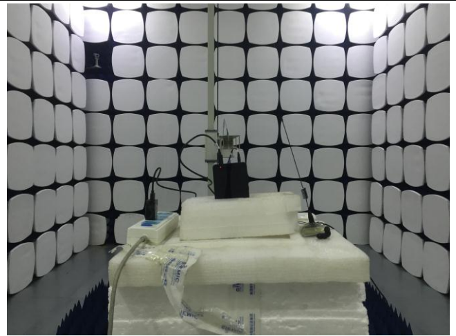
Radiated Spurious Emissions Test Setup Above 1GHz
