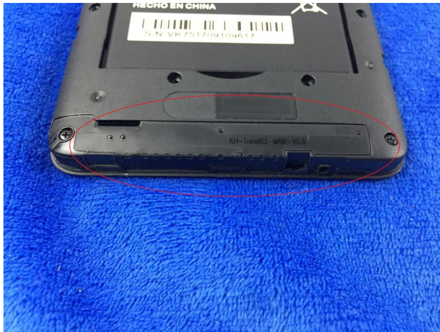
GSM/PCS/UMTS-FDD/LTE Antenna View
