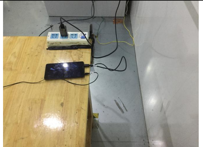
Conducted Emissions Test Setup Side View
