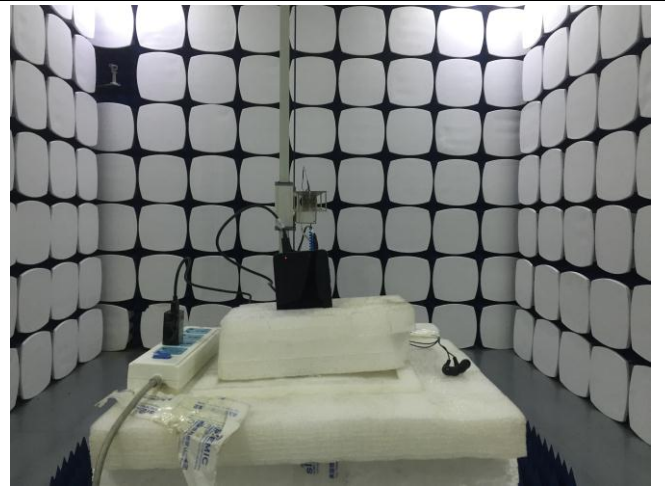
Radiated Spurious Emissions Test Setup Above 1GHz
