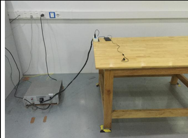
Conducted Emissions Test Setup Front View
