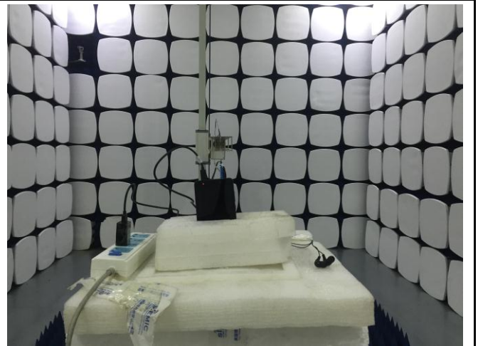
Radiated Spurious Emissions Test Setup Above 1GHz
