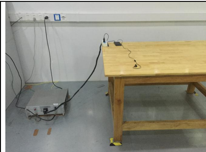
Conducted Emissions Test Setup Front View
