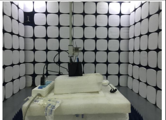
Radiated Spurious Emissions Test Setup Above 1GHz
