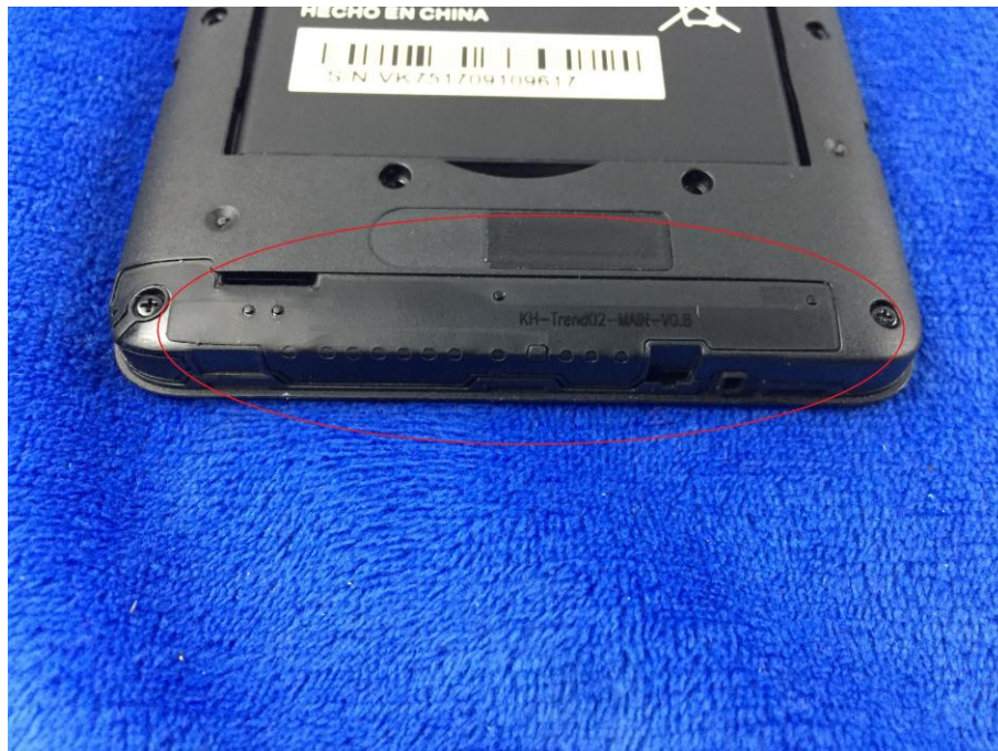
GSM/PCS/UMTS-FDD/LTE Antenna View
