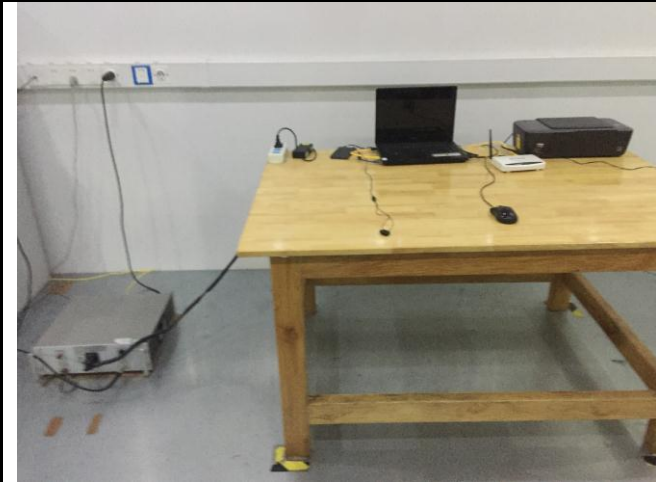
Conducted Emissions Test Setup – Front View
