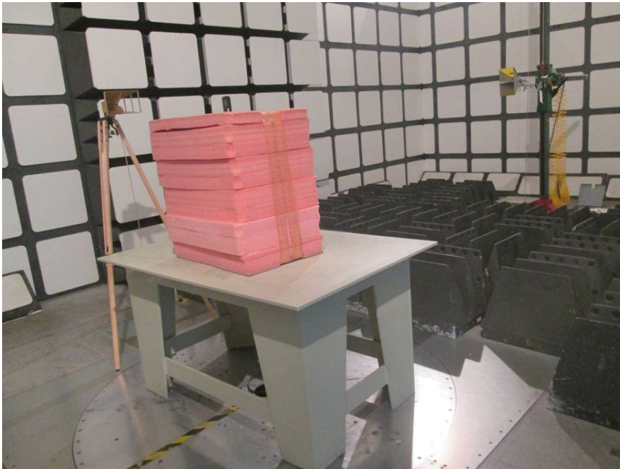
Radiated Emissions Test View (Above 1 GHz)
