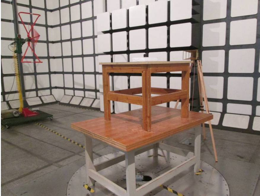
Radiated Emissions Test View (Below 1 GHz)
