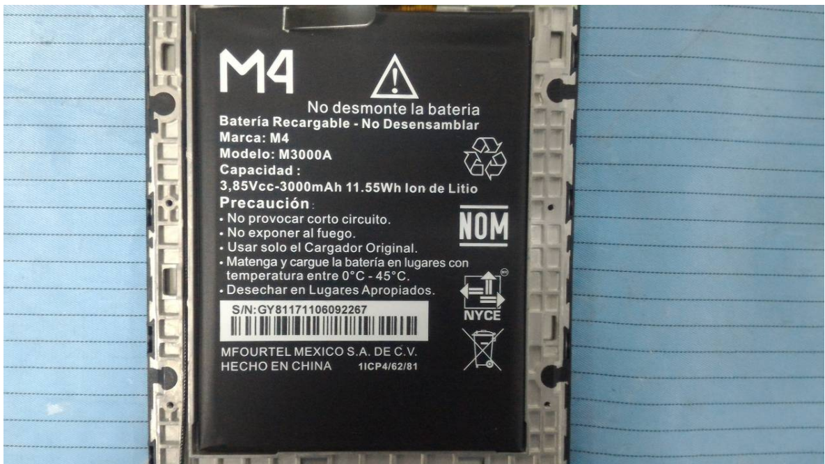
EUT – Battery label View
