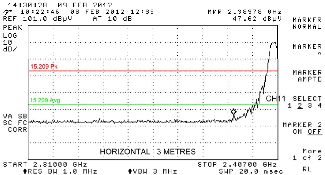
Bandedge CH11 2389MHz (Peak – Horizontal)
