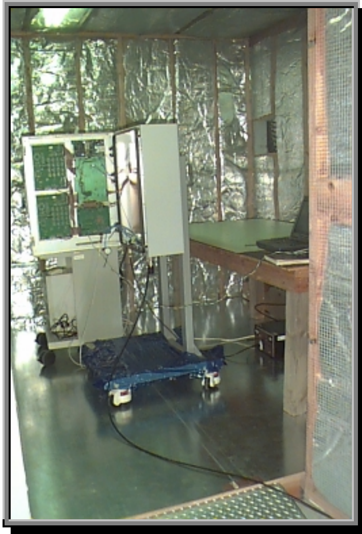
FCC Part 15.207 Conducted Emissions
