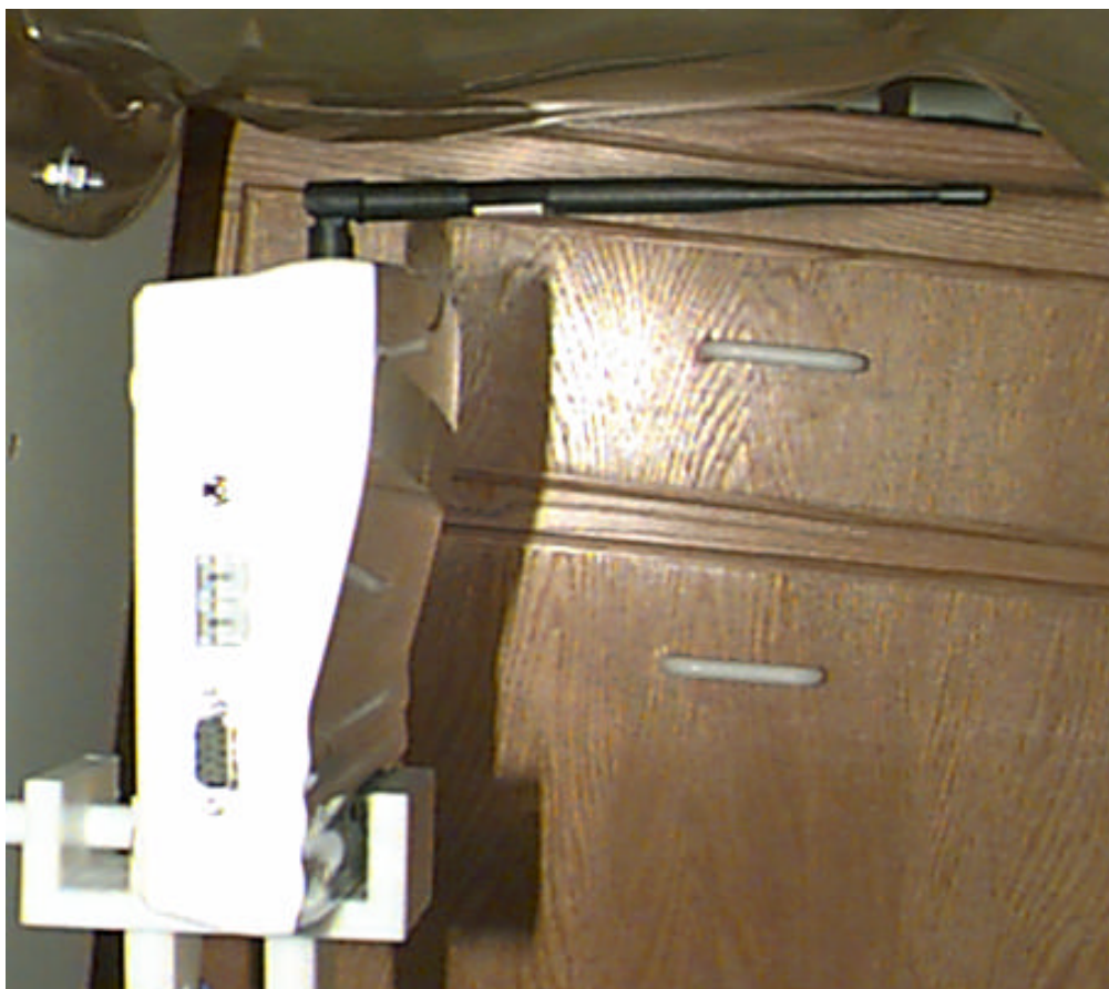
Figure 8. Test setup of EUT in normal operating position with the source of significant emissions (antenna) 3.0 cm below the phantom.
