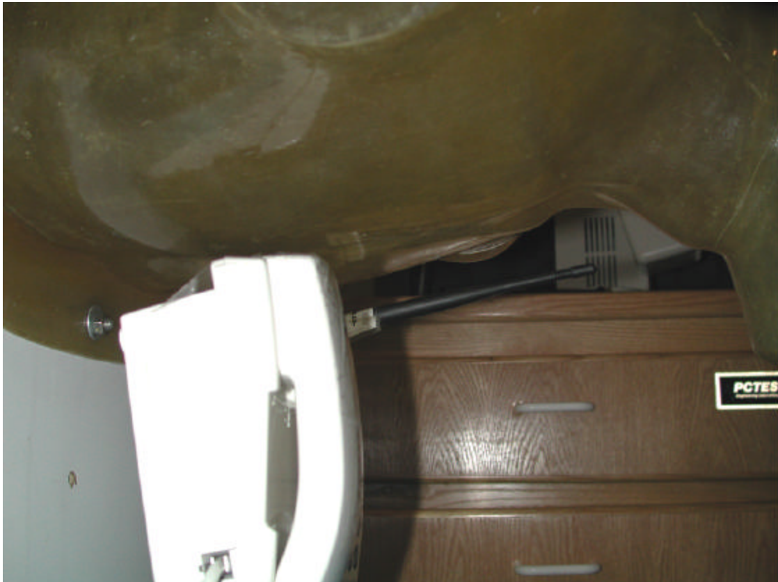
Figure 8. Test setup of EUT in normal operating position with the source of significant emissions (antenna) 2.5 cm below the phantom.
