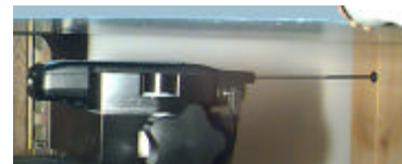
Figure 16. Body SAR Test Setup
