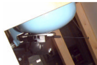
Figure 18. Head SAR Test Setup
