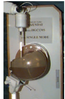
Figure 1. SAR Test Set-up
