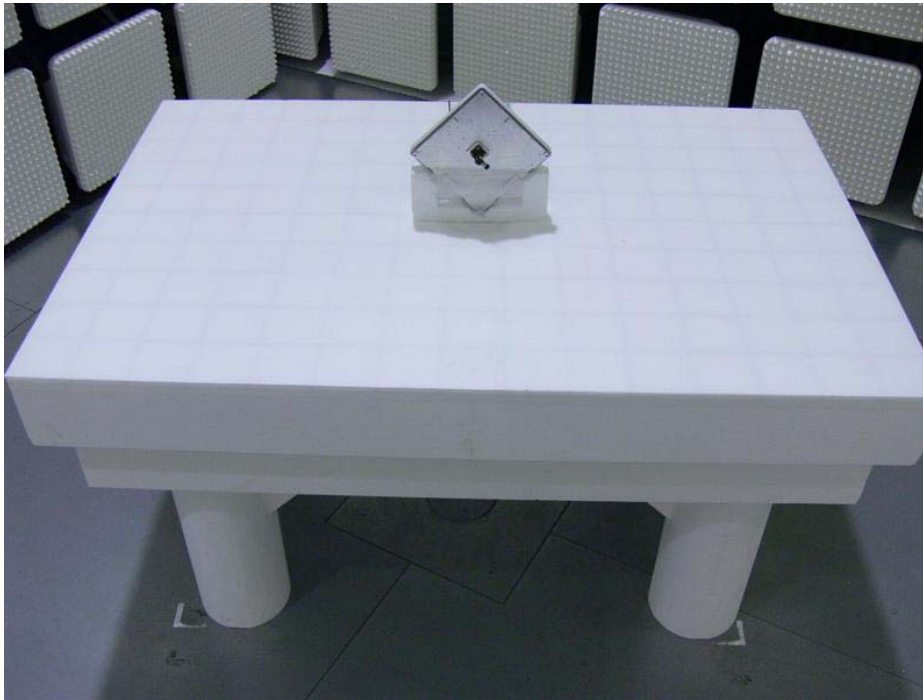
Photograph 4: Set-up for Radiated Emissions, Front View
