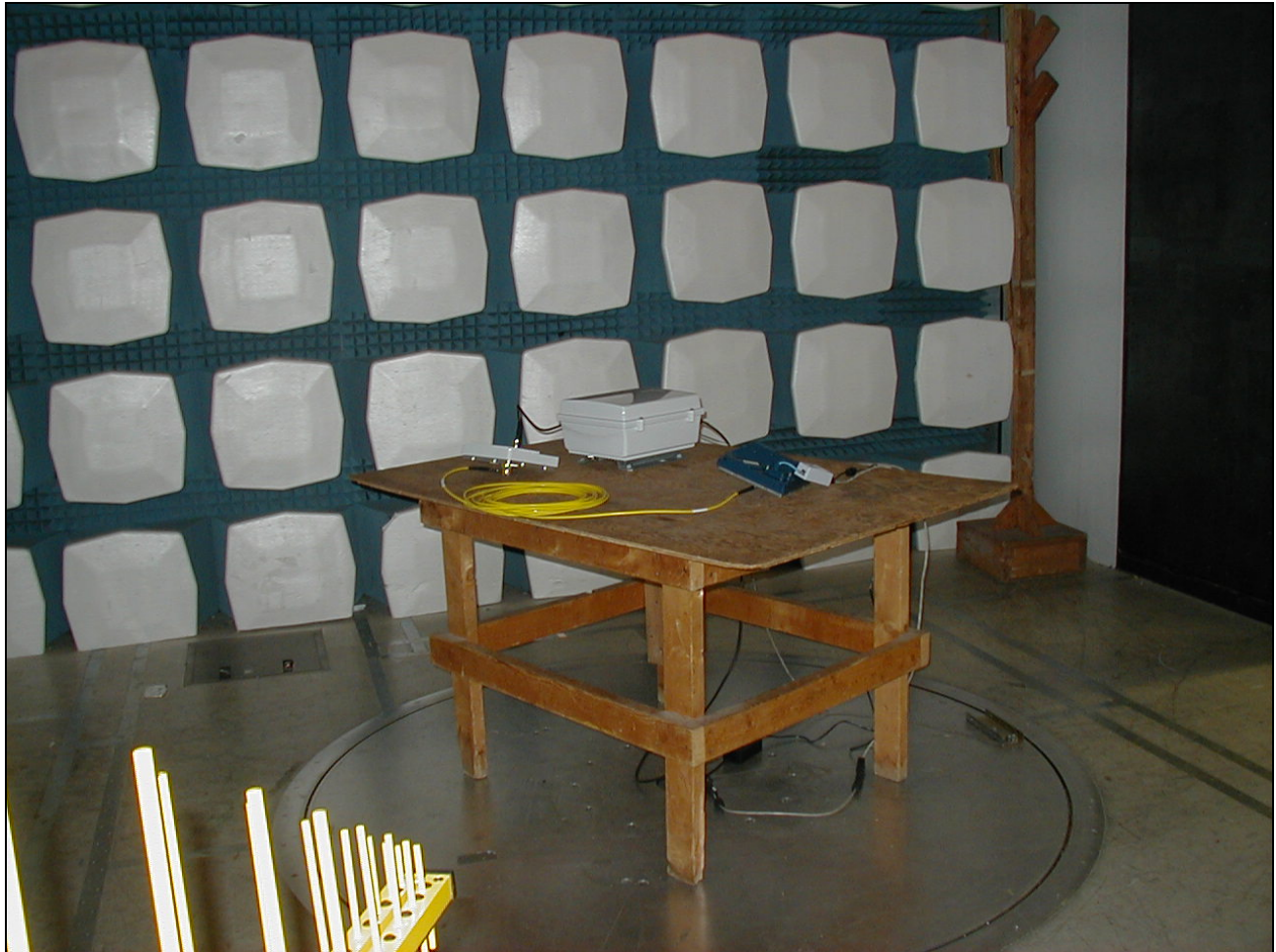
Photograph 2. Radiated Spurious Emissions, Test Set-up
