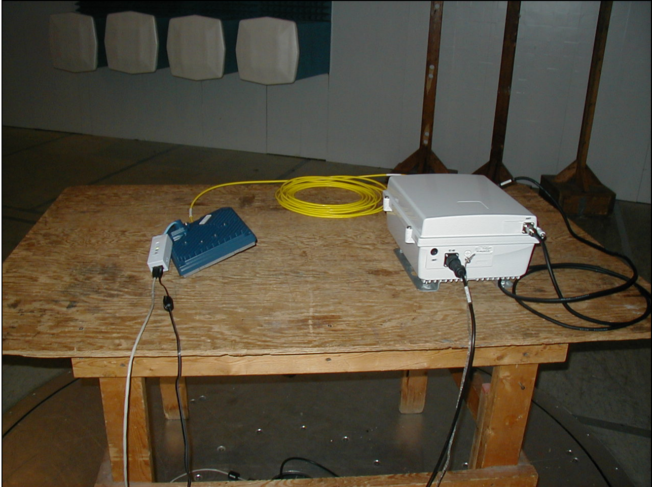
Photograph 2. Radiated Spurious Emissions Test Setup
