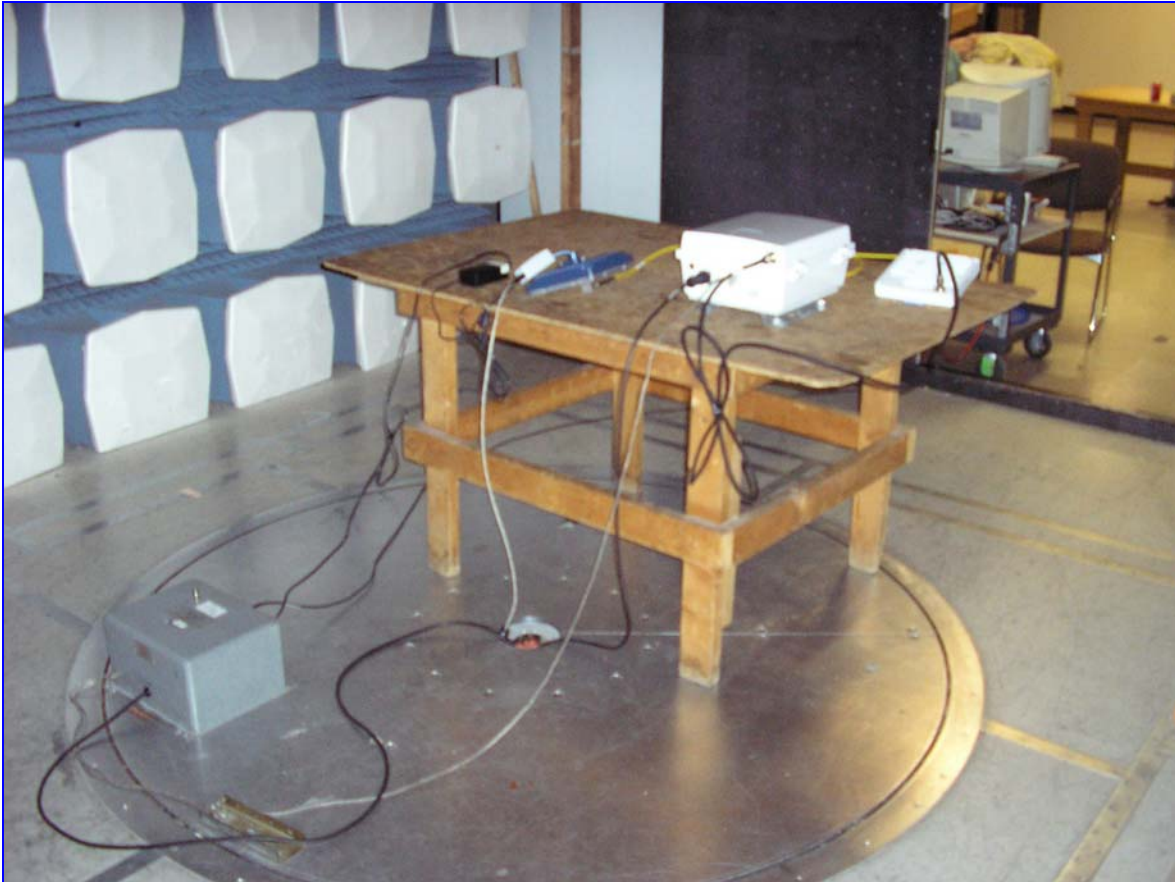
Photograph 1. Conducted Emissions Test Setup
