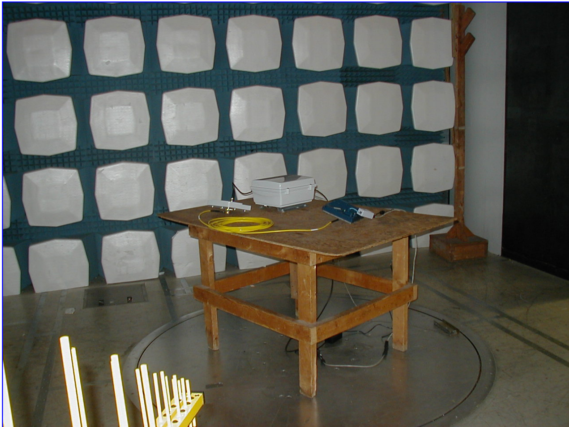
Photograph 3. Radiated Emission Limits Test Setup
