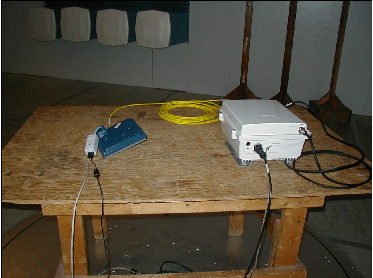
Photograph 2. Radiated Spurious Emissions Test Setup
