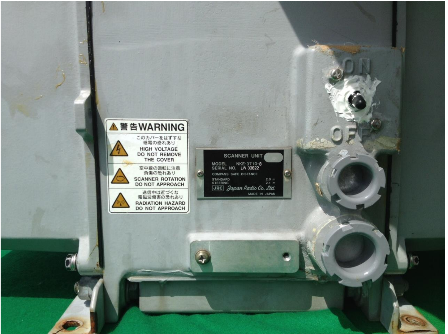
NKE-3710-8: Rear Side/cable insertion with Cover
