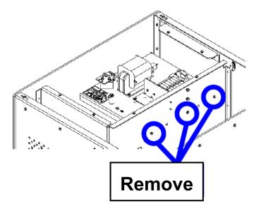
Remove the three screws (M4) that hold the modulation unit outside of the transmitter-receiver unit and the two bolts inside of the modulation unit.
