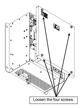
Step 3 Remove the cover of the T/R control circuit and replace the circuit.
