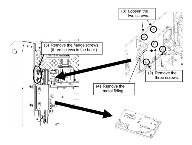
After having replaced the receiver, reassemble the unit by following the disassembly procedure in the reverse order. Do not forget to tighten the bolts or screws, and make sure that the cables are connected.
