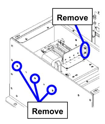
Remove the modulation unit together with the plate and replace the modulation unit. After replacing the modulation unit, reassemble the unit following the disassemble procedure in the reverse order. Make sure that there are no omissions of magnetron installation, bolt tightening, and cable connection.
