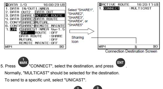
6. When "UNICAST" is selected, press and to select the destination IP "2.TO IP" and "3.PORT No.".
