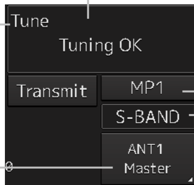
Solid state radar is connected as the radar antenna.
