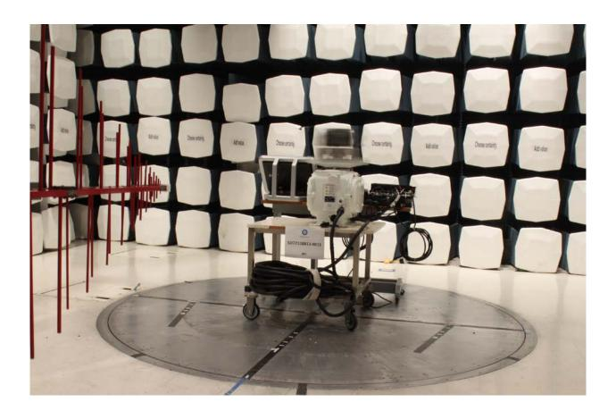
Radiated Emissions Test Setup (below 1GHz)
