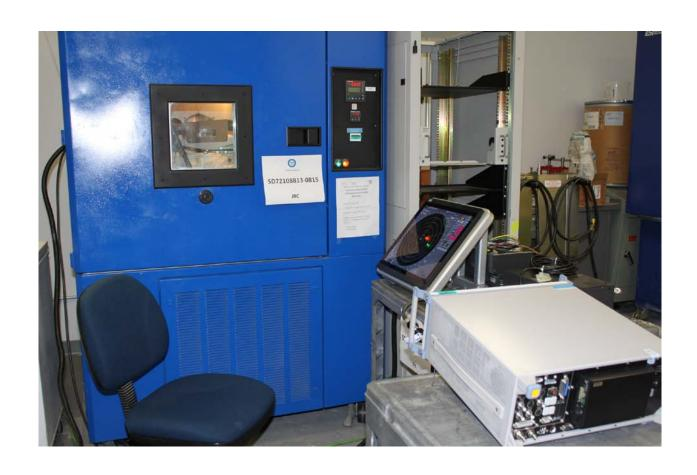
Frequency Stability Test Setup
