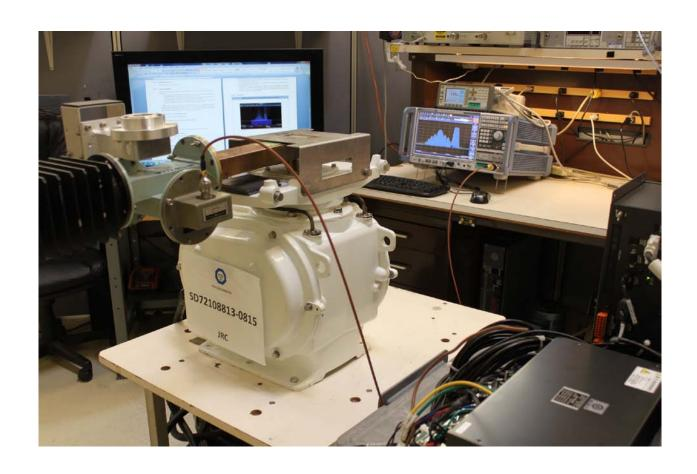
**Antenna Conducted Port Test Setup**
