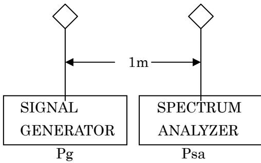
A signal source of known amplitude was used as a calibrating signal with identical antenna on the generator and the spectrum analyzer.
