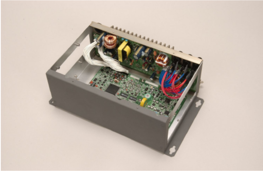
Inside of Processor unit.
