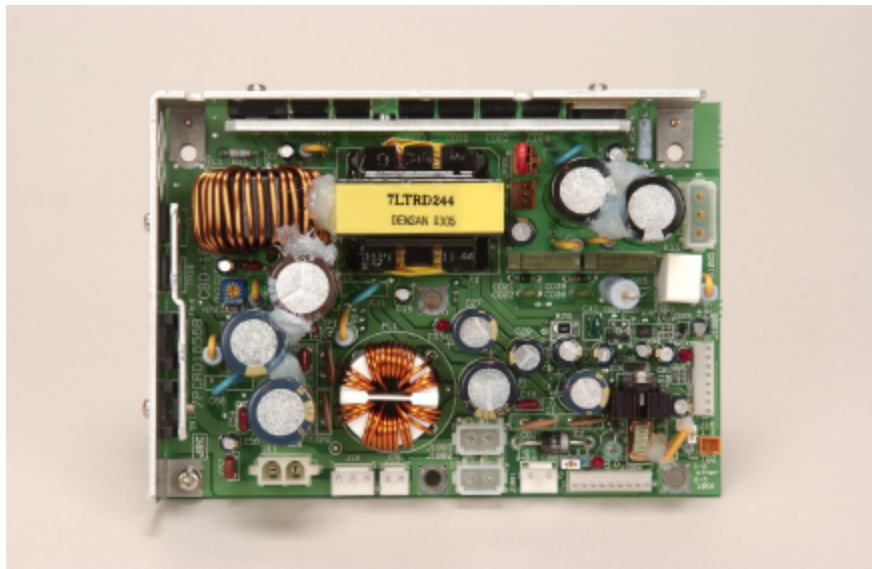
Power Supply Module Close up.
