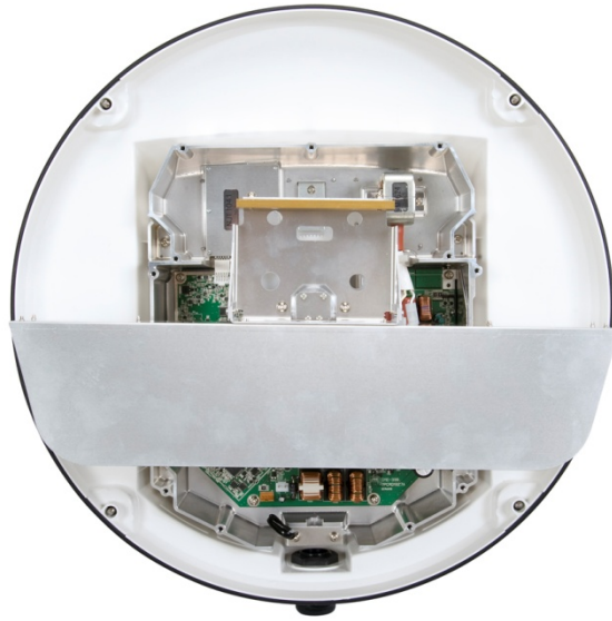
NKE-1066 without Radome, Cover for Waveguide
