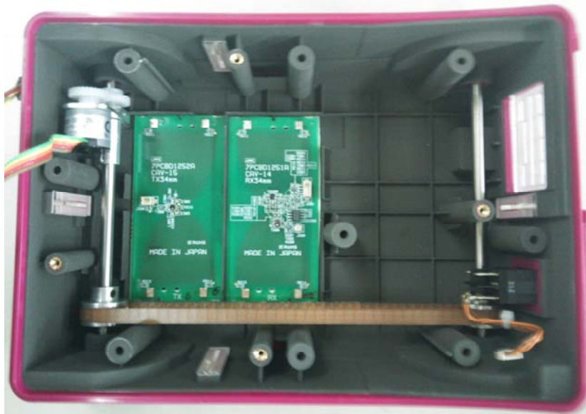
Figure 7 Antenna Circuit TX / Antenna Circuit RX
