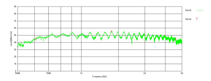
Center Frequency fC: 1391.156 MHz Lower boundary fL: 610.214 MHz Upper boundary fH: 2799.400 MHz 10dB Bandwidth: 1408.244 MHz
