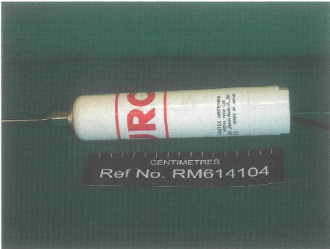
Figure 5: NAW-333 external view (whip length is 0.6m – not shown in photograph)
