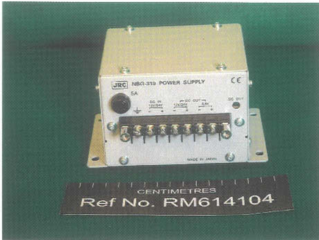
Figure 8: NBG-319 front view (terminal cover removed)
