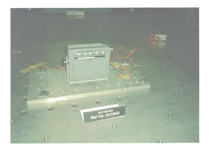
View No. 3 of NCR 330 during Vibration Test
