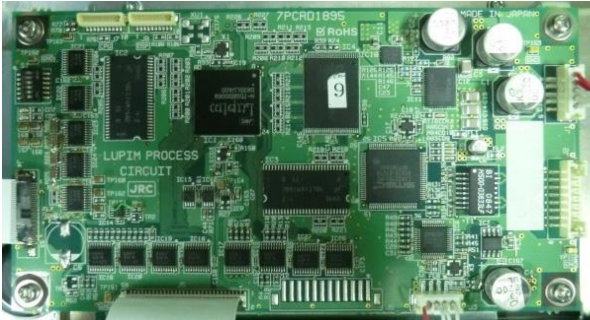
(18) CDC-1346B PROCESS CIRCUIT [NDZ-227 DATA TERMINAL]
