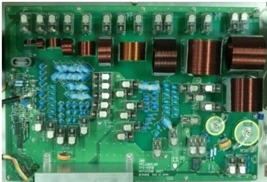
(11) CFG-2250 MATCHING UNIT [NFC-2250 ANTENNA TUNER]
