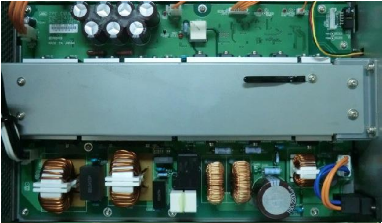
(8) CBG-2416 PA_PS UNIT [NBD-2250 POWER SUPPLY]
