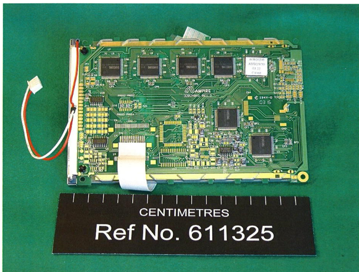
NCM-779 AIS Controller – Internal View 2
