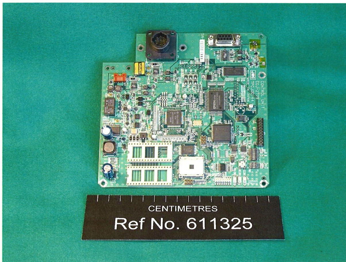
NCM-779 AIS Controller – Internal View 4
