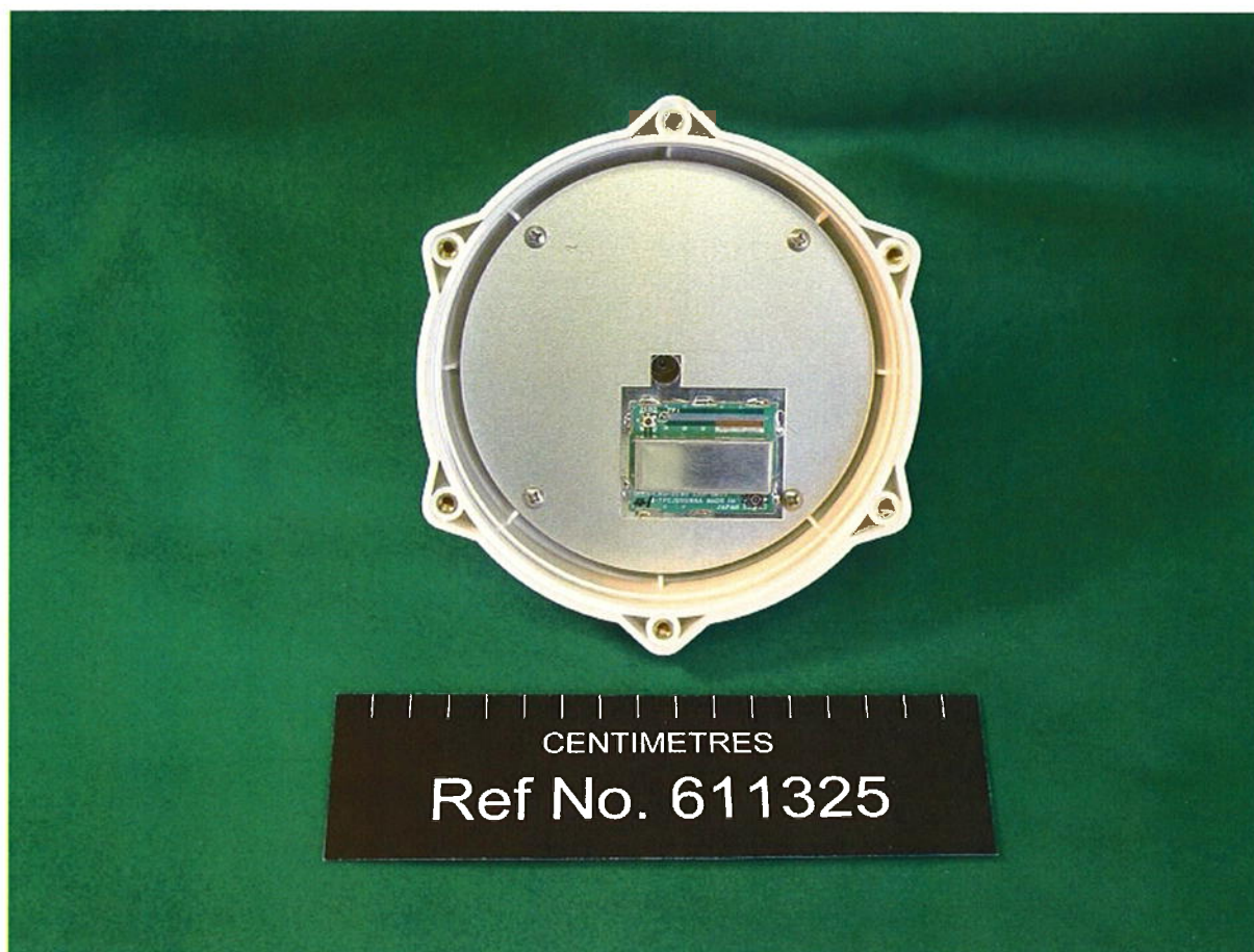
NTE-182 Transponder – Internal View 2
