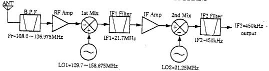
The first frequency converter circuit (1st MIX) mixes the received signal with the first local oscillator signal, whose frequency (LO1) is higher than the selected receive frequency (Fr) by the first intermediate frequency (IF1: 21.7 MHz), to down-convert the received signal to the first intermediate frequency band (Fr to IF1).
