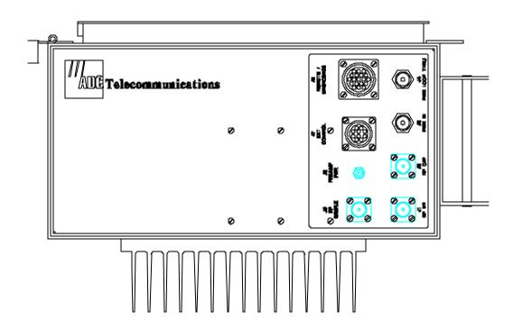
**RF I/P (J1)** Provides an RF input to the unit
