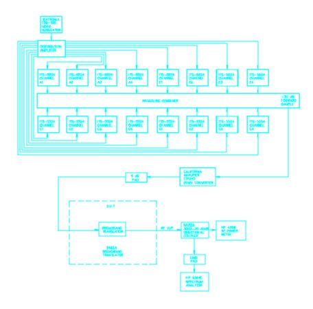
Before testing the 6452A multi-channel translator, the ITS-5724 transmitters (FCC ID# CJJ79SITS-7022) used to generate the multi-channel input signal to the translator were tested and observed to meet specifications. Then, the translator was tested and observed, as illustrated in the following sections, to reliably reproduce the transmitted signals in acordance with the rules set forth in the Rules and Regulations.
