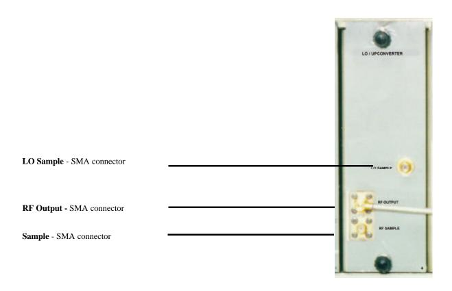
This module consists of the A1, LO/ Upconverter board, a channel filter, and an output amplifier board. This module takes an external IF and converts it to the final RF output frequency using an internally generated local oscillator.
