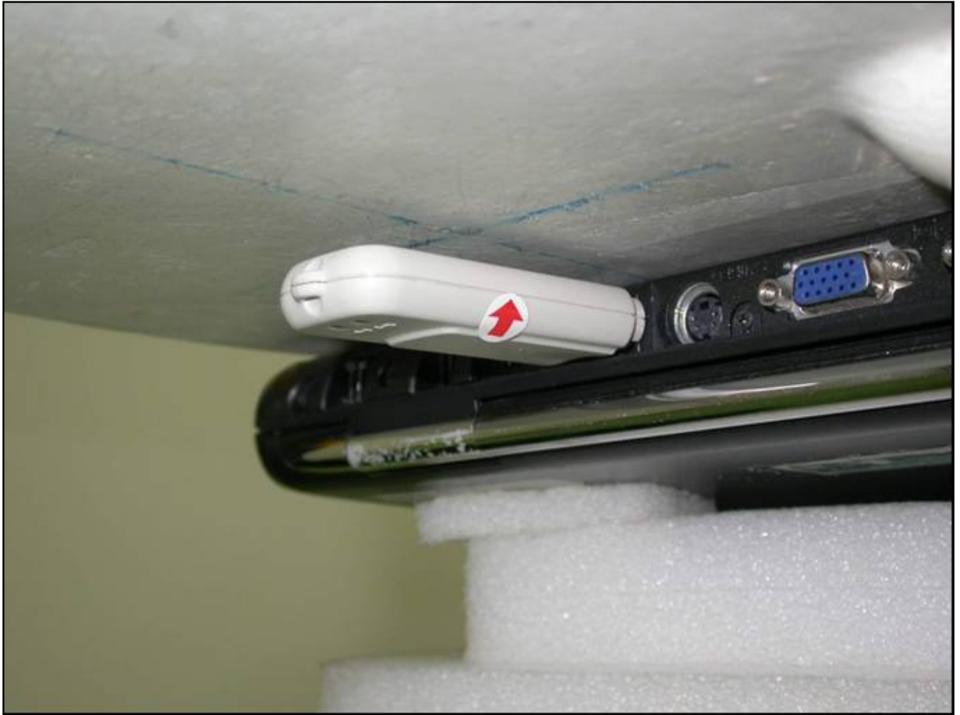
The bottom of the EUT to the flat phantom distance 8 mm
