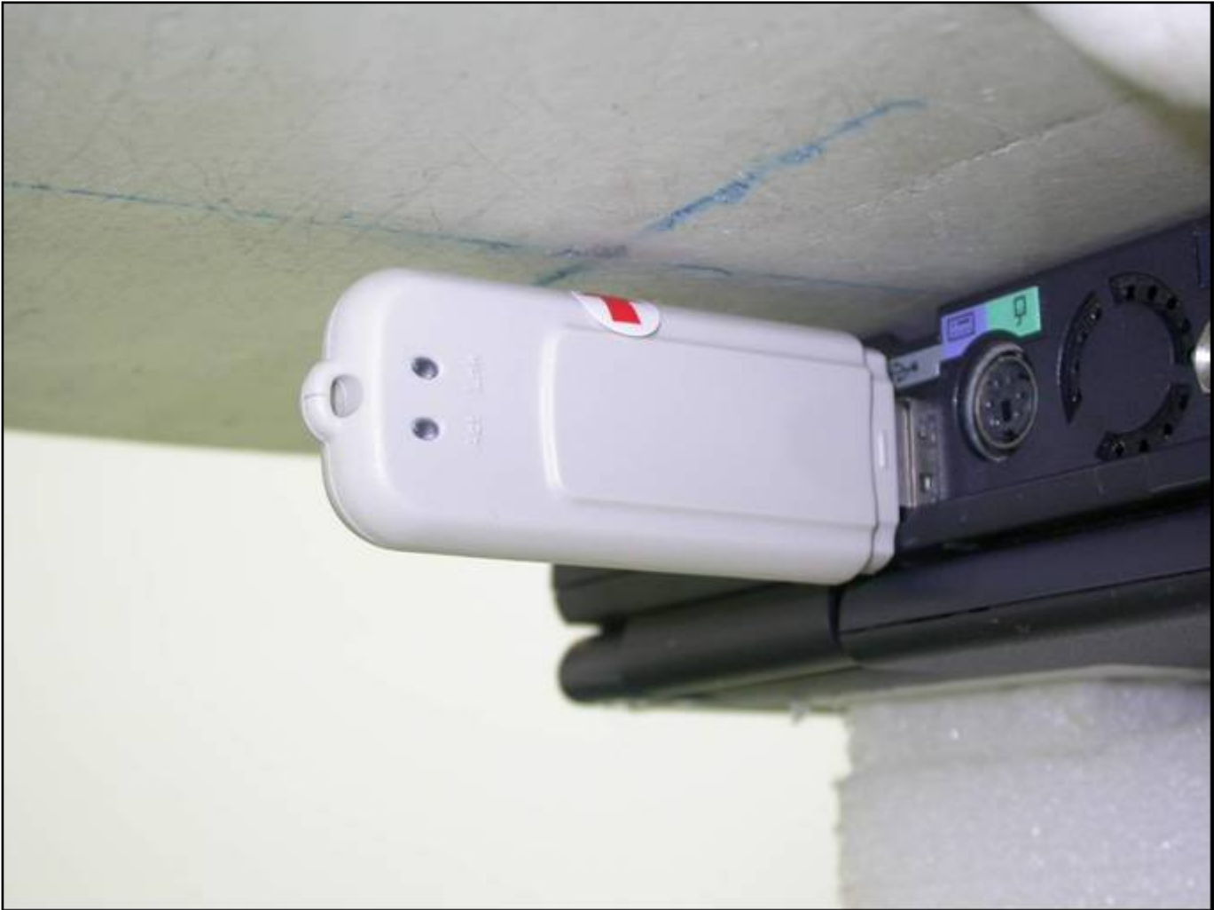
The edge of the EUT to the flat phantom distance 5 mm
