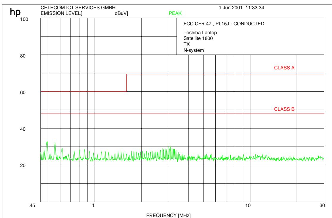
The test was performed with a CISPR quasi peak adapter.
