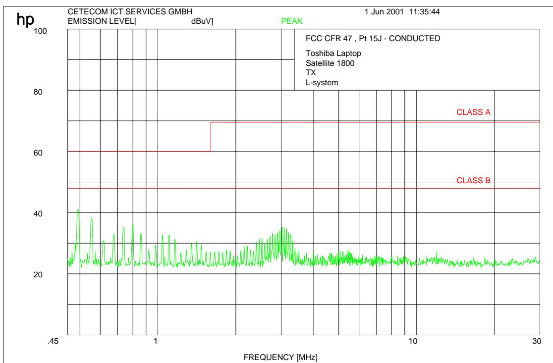
**The test was performed with a CISPR quasi peak adapter.****All spurious were below limit.****Technical specification : 15.207 (Revised as of October 1, 1991 )****Limit**
