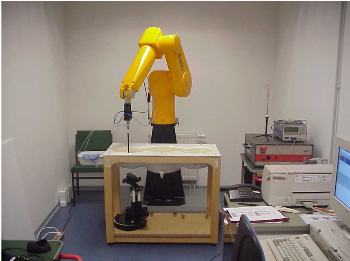
Photo 1: Measurement System DASY 3
