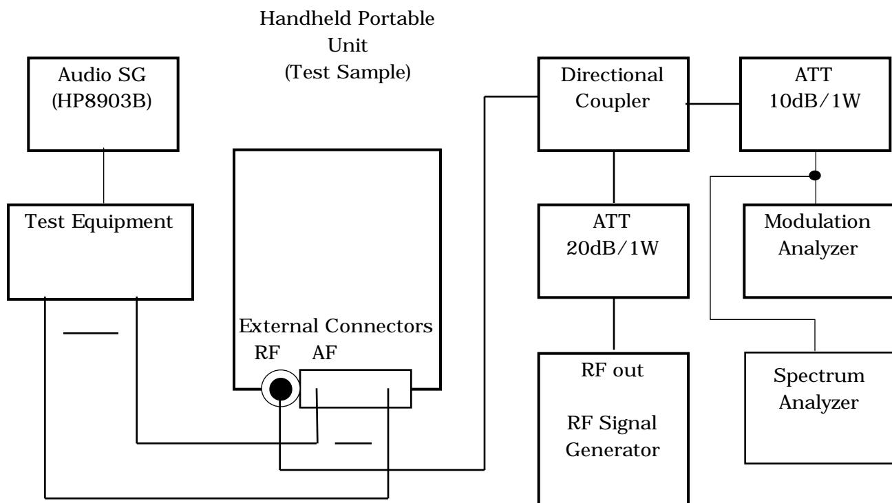
TRANSMITTER TEST SET-UP (2)
