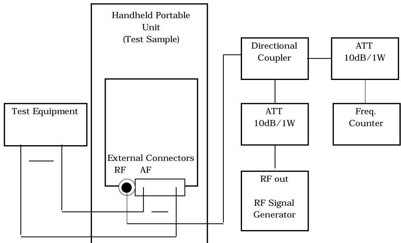
TRANSMITTER TEST SET-UP (3)
