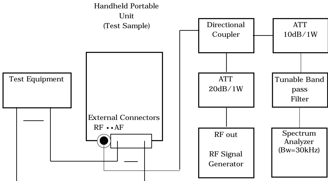
TRANSMITTER TEST SET-UP (4)
